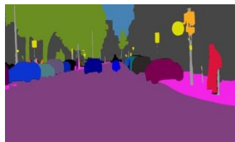
Panoptic segmentation results of the EfficientPS network, proposed by ALU-FR
