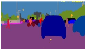
Panoptic segmentation results of the EfficientPS network, proposed by ALU-FR
