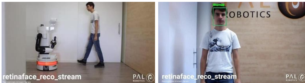
OpenDR toolkit code running in the Jetson TX2 embedded in TIAGo.
