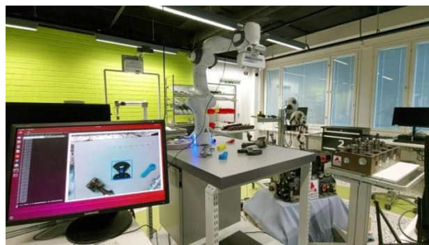
Agile production use case scenario combining the single demonstration object grasping model and the speech recognition model.
