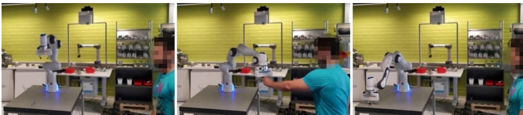
Different stages of the hand-over scenario by speech command-based coordination.
