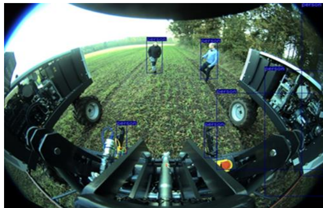
Human detection example on an image collected from the Robotti platform. Both true and false detections are evident, highlighting the need to adapt existing models to the particularities of agriculture use case.
