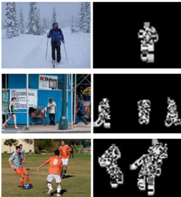
Heatmaps generated as part of the active efficient high resolution pose estimation approach proposed by AUTH.
