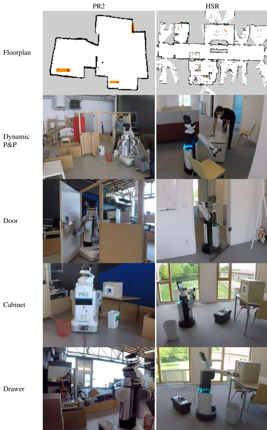
Fig. 5. Real world experiments on the PR2 (left) and HSR (right) robots. From top to bottom: environment map, pick&place while avoiding static and dynamic obstacles (table locations marked in orange), opening and driving through a door, opening a cabinet and opening a drawer with static obstacles constraining the base.
