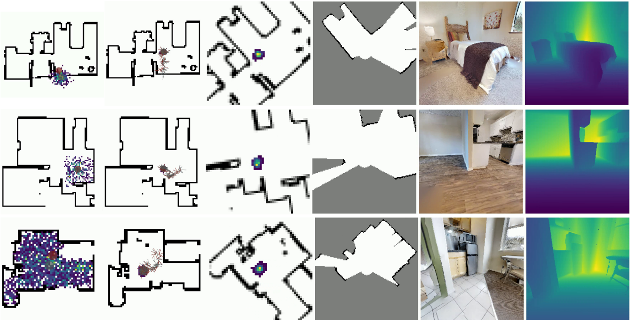
Fig. 3: Examples for the tracking (top), semi-global (mid) and global (bottom) localization tasks. Left: the initial particle distribution, second from left: the global map and trajectory of the agent. Green arrows denote the estimated poses and red the ground truth poses at each step. Circles denote the final estimated and ground-truth poses. Third from left to right: the local belief map observed by the RL agent, the current observations: occupancy grid, RGB and depth.
