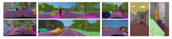
Fig. 5. Qualitative performance of our pseudo-label generator in four diverse domains from both public and in-house data sources. From left to right, we show Cityscapes [4], KITTI-360 [15], in-house automated driving, and an in-house office environment.
