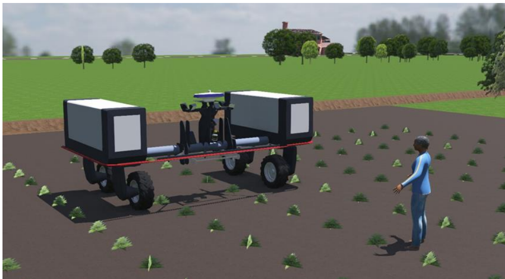
Figure 8: Robotti robot operating on a field and detecting the presence of humans.
