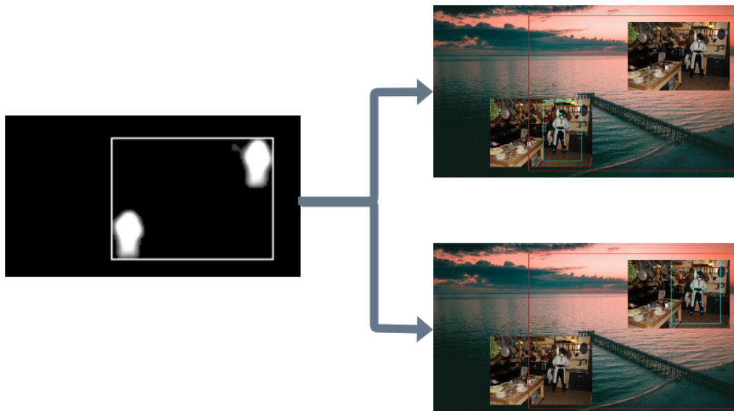
Figure 5: An example of applying the proposed ROI extraction approach. Note that instead of extracting one global ROI (red bounding box) - as done in the previous approach described in D3.3, we extract two smaller ROIs (cyan bounding boxes). This enables processing the input image faster since a smaller portion of it needs to be analyzed in high resolution.
