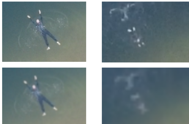
Figure 14: Effects of down sampling the images taken from different altitudes
