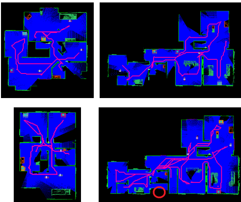
Fig. 3. Example trajectories of HIMOS in unseen apartments. Black: unexplored, blue: free space, green: walls, red: agent trace, grey: (found) target objects, other colors: miscellaneous objects. Bottom right: the agent failed to find the last object, marked by the red circle, in the given time.
