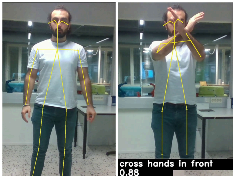
Figure 4.2.1: Human skeleton detection skeleton-based tracker Lightweight OpenPose. Recognized action is 'cross hands in front', with its corresponding confidence score.
