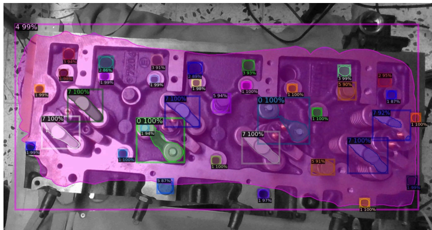
Figure 4.4.1: The image depicts detection of targets (five classes): rocker arm location (class 0), bolt holes (class 1), big and small pushrod holes (class 2 and 3) and engine (class 4). Each detection is labeled with the detected class and their corresponding confidence score.
