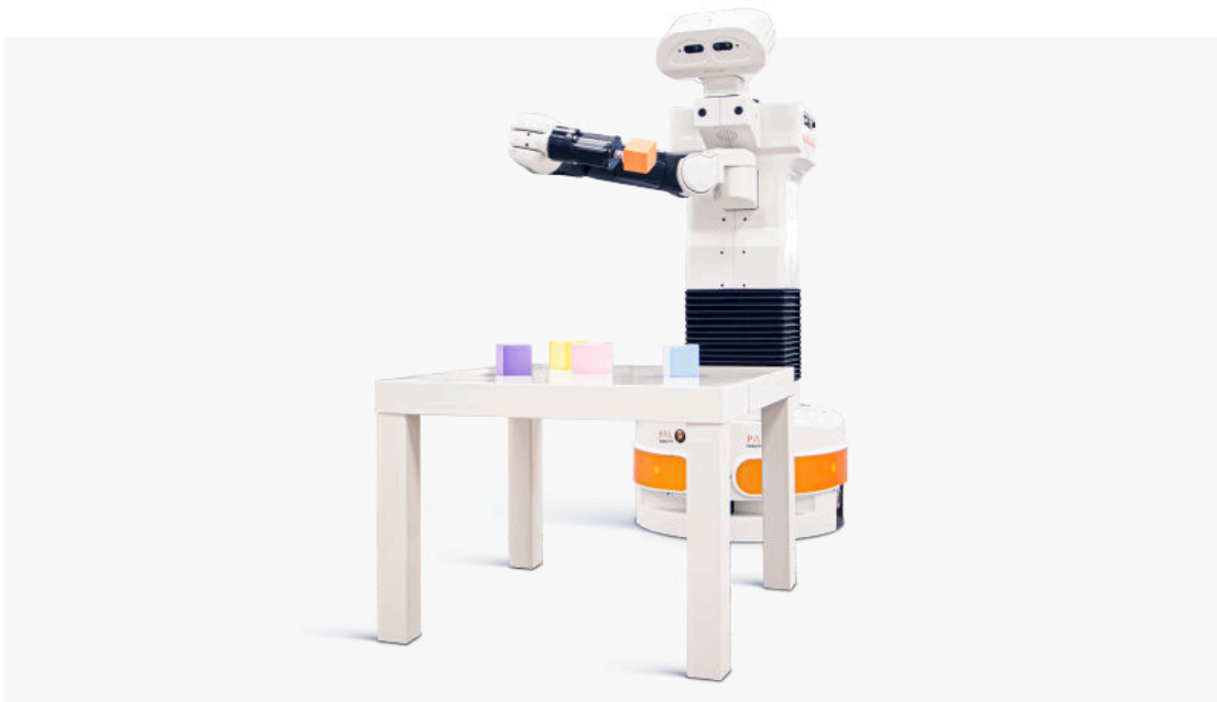
Figure 3.2.1: TIAGo grasping an object using the Advanced Grasping package
