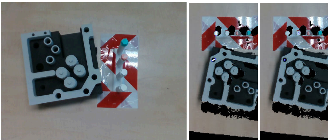
Figure 4.10.2: PARTNR Tool Demonstration for Robotic Pick-and-Place Task. Left: Input image to PARTNR depicting initial task setup. Middle: Operator demonstration of the desired action. Right: Automated pick-and-place action proposed by PARTNR after interactive training phase. This sequence illustrates the progressive autonomy of the robotic system using PARTNR, which reduces the need for extensive pre-training by employing operator demonstrations to rapidly refine the policy, thus enhancing trustworthiness and minimizing operator disruptions.
