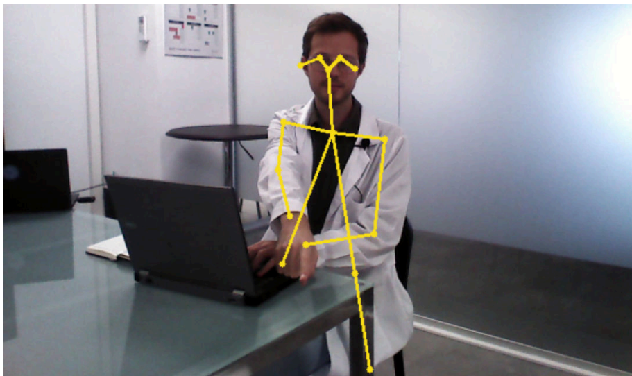
Figure 3.2.3: skeleton detection: pointing at bottle
